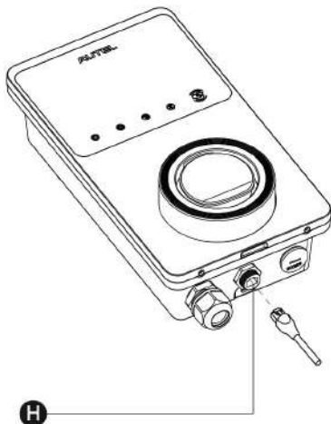
Figure 3-6 Plugging the RJ45 Cable
