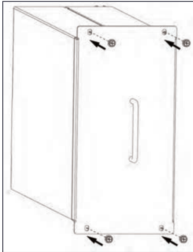
Figure 5-26 Installing the Filler Module
