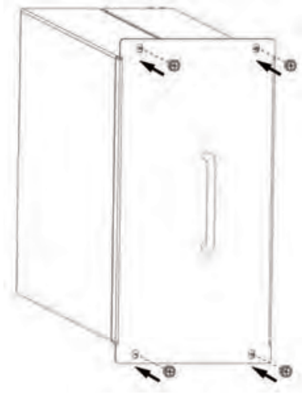
Figure 5-25 Installing the Filler Module
