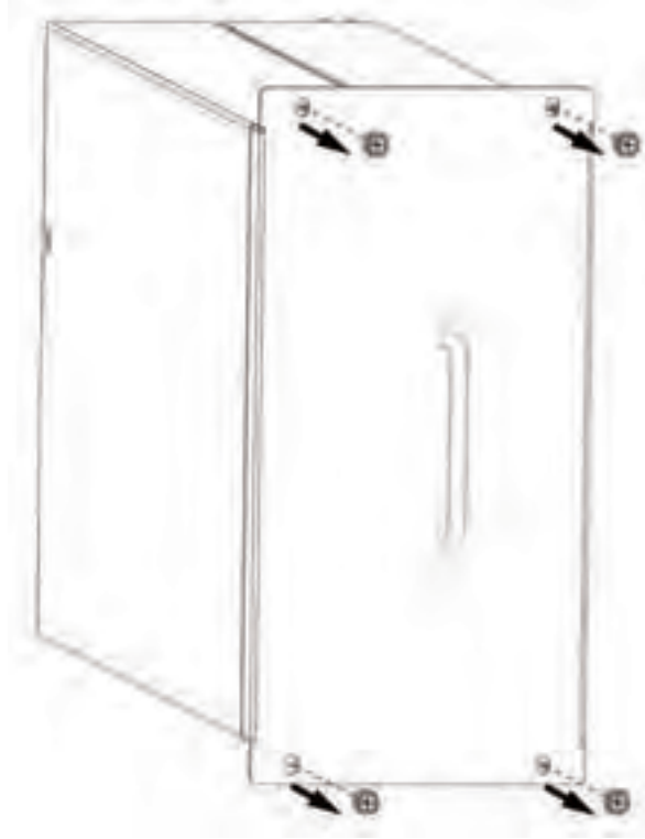
Figure 5-22 Removing the Filler Module
